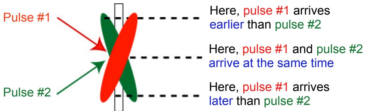
Fig. 3a. Crossing beams at an angle maps delay onto transverse position.
