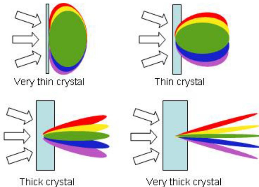
**Fig. 4.** Thin and thick SHG crystals illuminated by converging broadband light and polar plots of the generated colors vs. crystal exit angle. Note that the very thin crystal (ordinarily required in pulse-measurement techniques) generates the second harmonic of all colors in the forward direction. The very thick crystal, on the other hand, does not and, in fact, acts like a spectrometer. The thick crystal thus acts like a thin crystal *and* a spectrometer.
