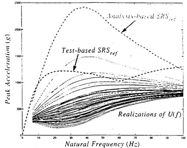
Figure 11: Analytically-based reference SRS.
