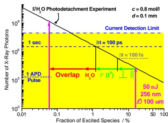
**Fig. 4:** Required number of incident x-ray photons to observe a pump-probe signal in the iodide photodetachment experiment for 0.8 mol/l concentration and sample thickness 0.1 mm.
