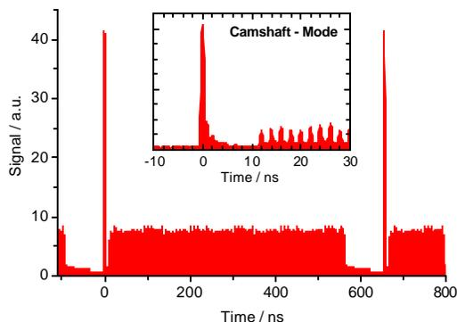
**Figure 1:** Oscilloscope trace from a fast photodiode recording visible light available at beamline 5.3.1 for timing and synchronization purposes.
