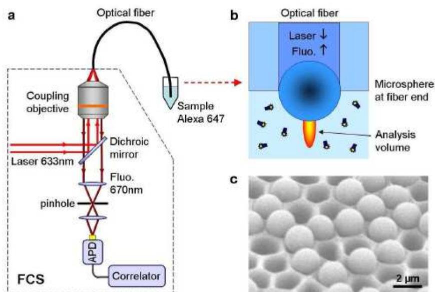
**Fig. 1.** (a) experimental setup, (b) end of the optical fiber with the microsphere, (c) electron microscope image of the optical fiber bundle etched with polystyrene microspheres.
