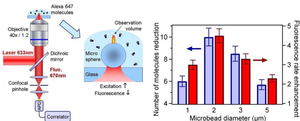
**Fig. 1:** Left: Schematic view of the experimental setup. Right: observation volume reduction and fluorescence rate enhancement versus microsphere diameter.
