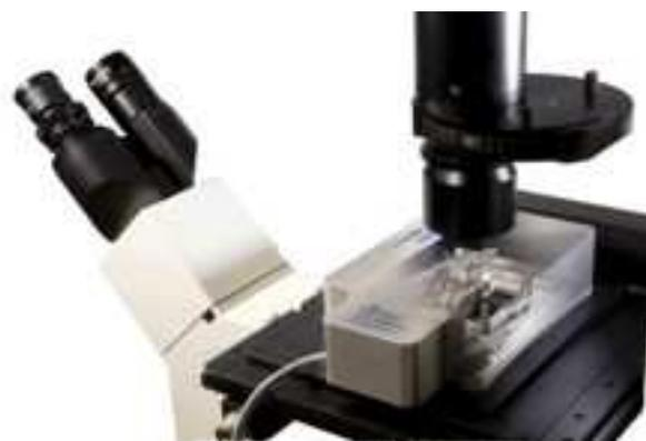
**Fig. 2.** Detection unit of the Ionovation Bilayer Explorer (Photoart) with a fully automated liquid handling and perfusion unit on a standard inverted microscope.
