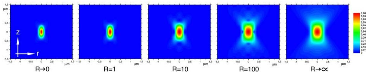
**Fig. 1.** Calculated observation volume for different values of the laser excitation (a scalar approach was used, as describe in [3]).  $R$  is the ratio of the laser excitation  $I_e$  to the saturation intensity  $I_s$ ,  $R = I_e/I_s$ .
