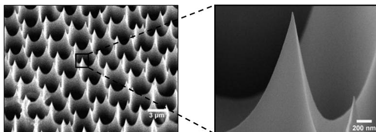
**Fig. 1** Scanning electron micrographs of a part of the nanotip array
