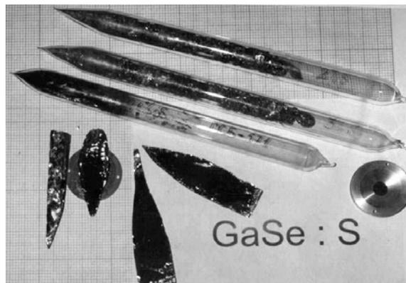
Fig. 1. Ampoules with synthesized compound, cleaved crystals and an optical element (Siberian Physico-Technical Institute, Materials Science Laboratory)
