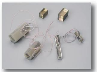
To compensate for natural birefringence the pair of identical LT elements with orthogonal Z- axis orientation is used in LT Q-switch design. Input and output edges (XZ planes) are equipped with antireflection coatings, YZ-planes are covered with metal films for electric field application. Lithium tantalate Q-switches may be used both in quarter-wave and half-wave schemes. Specifications of LT Q-switches are presented in table.
