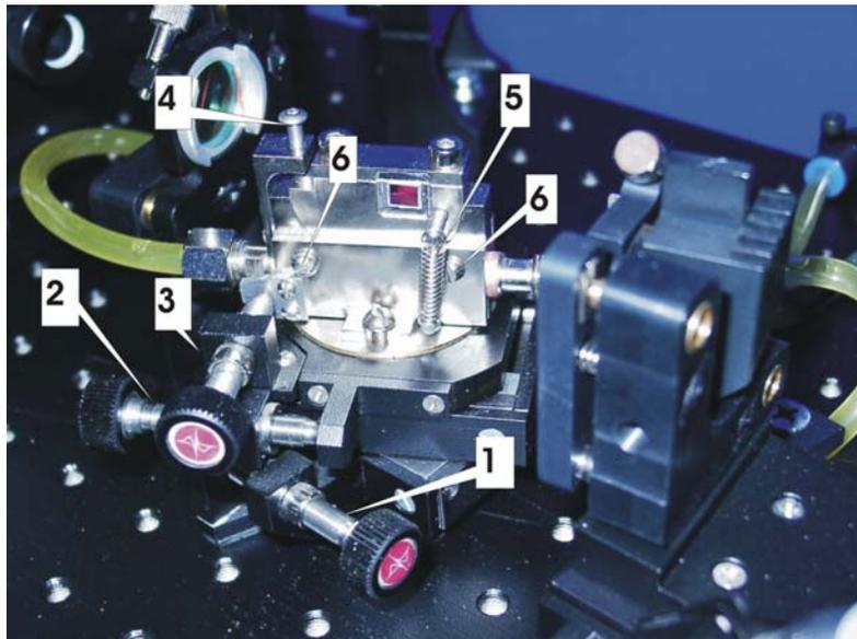
1. Screw for aligning crystal position on optical axis. 2. Screw for transverse aligning. 3. Screw for aligning Brewster angle. 4. Screw for aligning crystallographic axis orientation. 5. Spring
