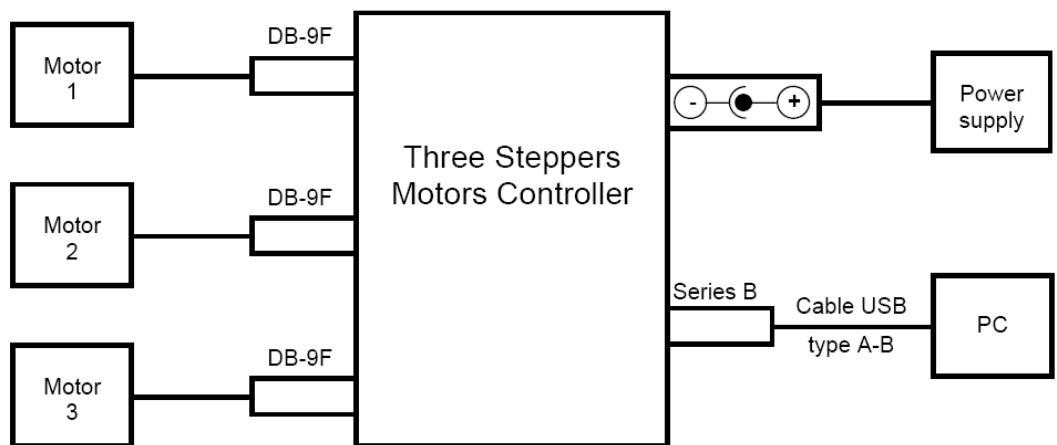
*Fig. 18 Connection scheme of the Three motor Controller*
