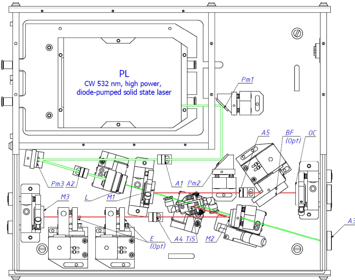
*Fig. 4 Schematic setup of the Trestles-CW*
