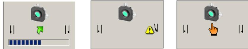
Motor motion      Limit switch closed      Manual mode
