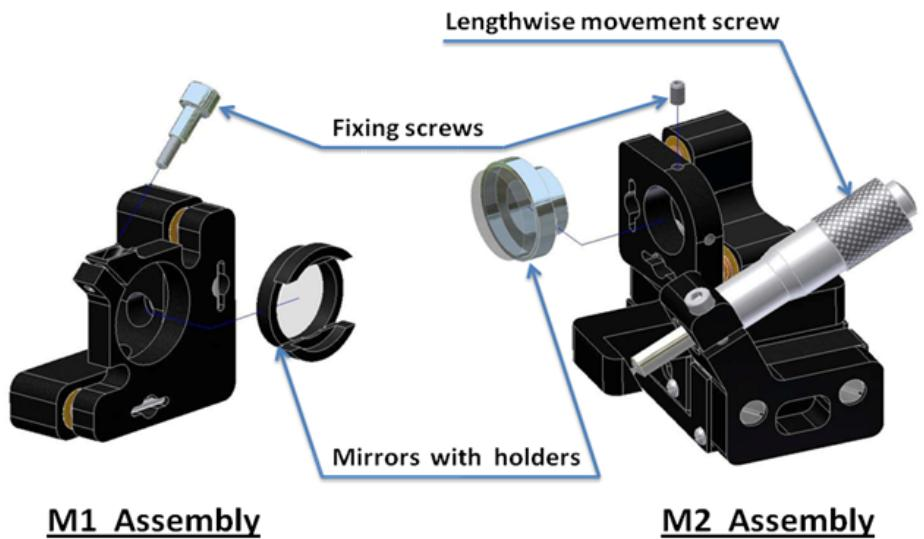
*Fig. 6 M1 and M2 assembly*
