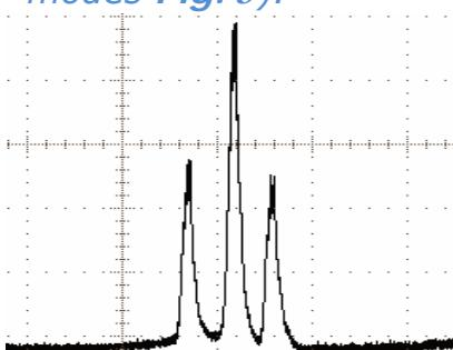
**Fig. 5 Oscilloscope image obtained by Fabry-Perot scanning interferometer (3 longitudinal modes).**
