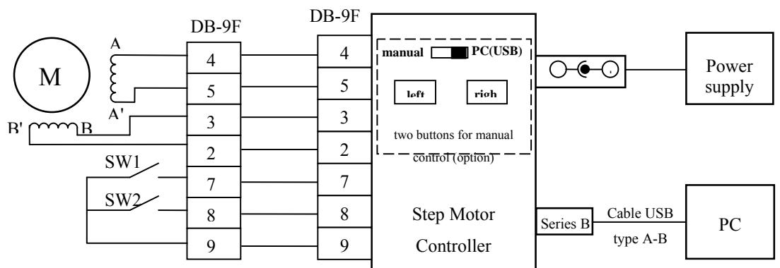
*Fig. 17 Connection scheme of the Single motor Controller*
