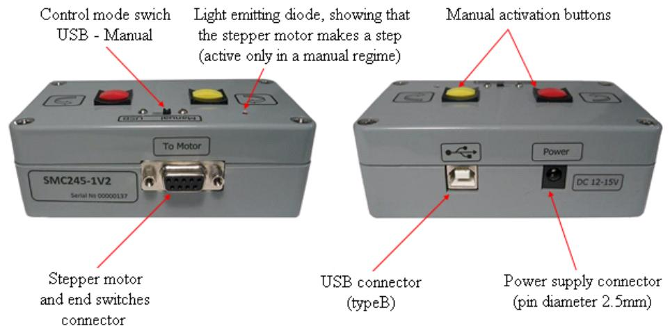
***Fig. 16 Outside view of the Single motor Controller***
