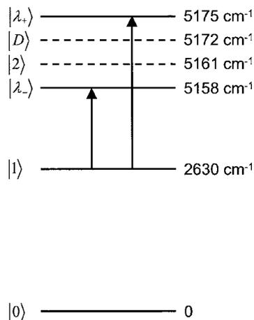
FIG. 6. Energy-level diagram for 2MP in  $\text{CCl}_4$ . The arrows indicate the transition eigenstates (solid lines) that give rise to the doublets in the 1-2 transition regions of the 2D correlation spectra in Figs. 3(a) and 3(b). The dashed lines represent the basis states.
