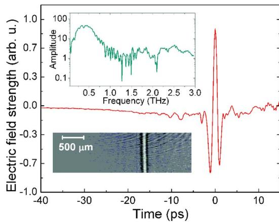
FIG. 2. (Color online) Temporal profile and spectrum of the terahertz pulse, determined from the grayscale image shown.
