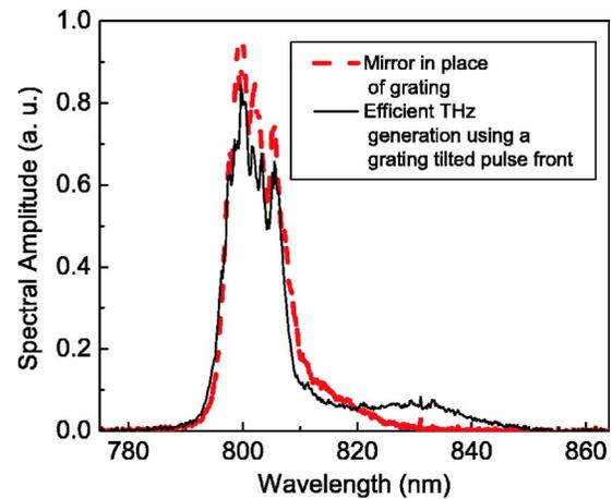
FIG. 3. (Color online) Spectra of the pump pulses scattered from the LN crystal with optimized (solid curve) and reduced (dashed curve) terahertz generations.
