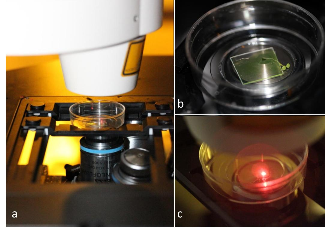
Figure 1. Overview of optoperforation setup optimized to minimize root damage and be consistently repeatable. (a)Confocal microscope stage with 15mm glass-bottom dish (MatTek<sup>®</sup>). (b) Arabidopsis thaliana orientation in the dish, immersed in a PBS-dextran solution, covered with plastic coverslip, mounted on 40X objective. (c) Focused femtosecond pulse of 700nm wavelength laser, aimed at the wall of a single root cell.
