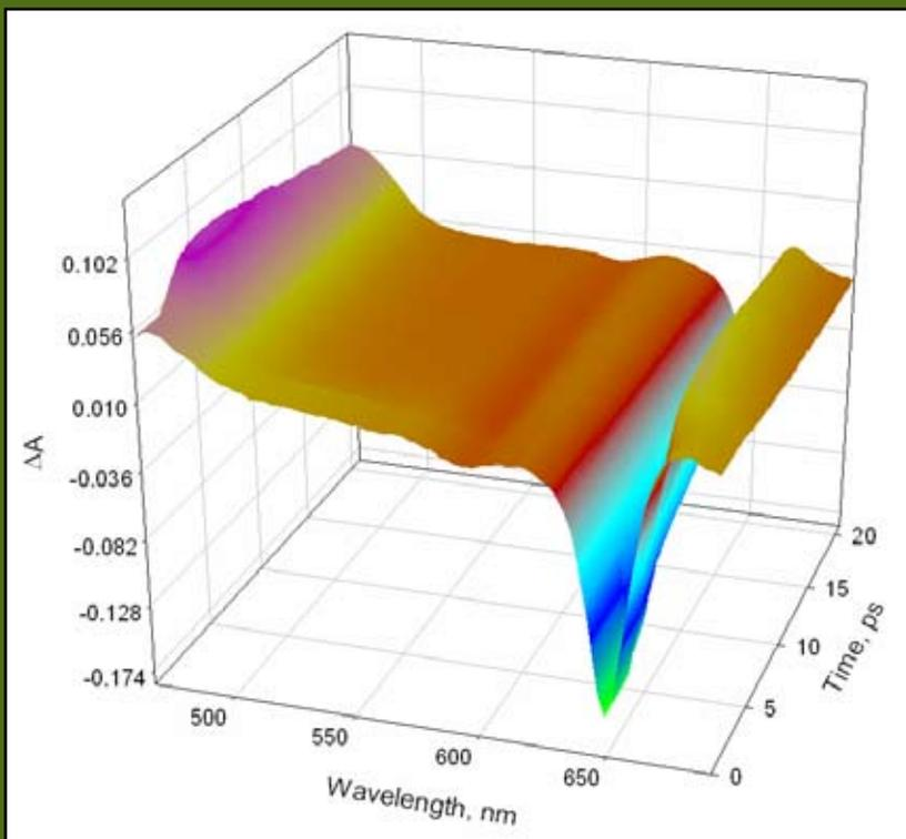
Three-dimensional diagram depicting time-resolved transient absorption for Ni(II) tetraphenyltetrabenzoporphyrin (NiTPTBP) in benzene.
