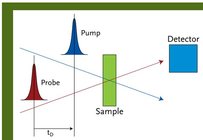
For time resolved pump-probe experiments two independently tunable and synchronized pulses are needed.
