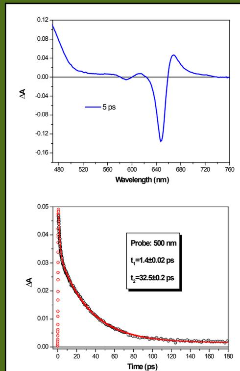
Transient spectrum at 5 ps. (Top) Kinetic profile at 500 nm. (Bottom)
